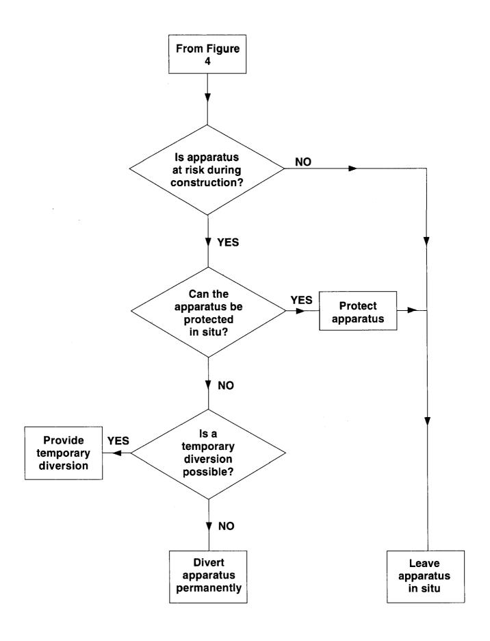
FIGURE 3 APPARATUS AT RISK DURING CONSTRUCTION
